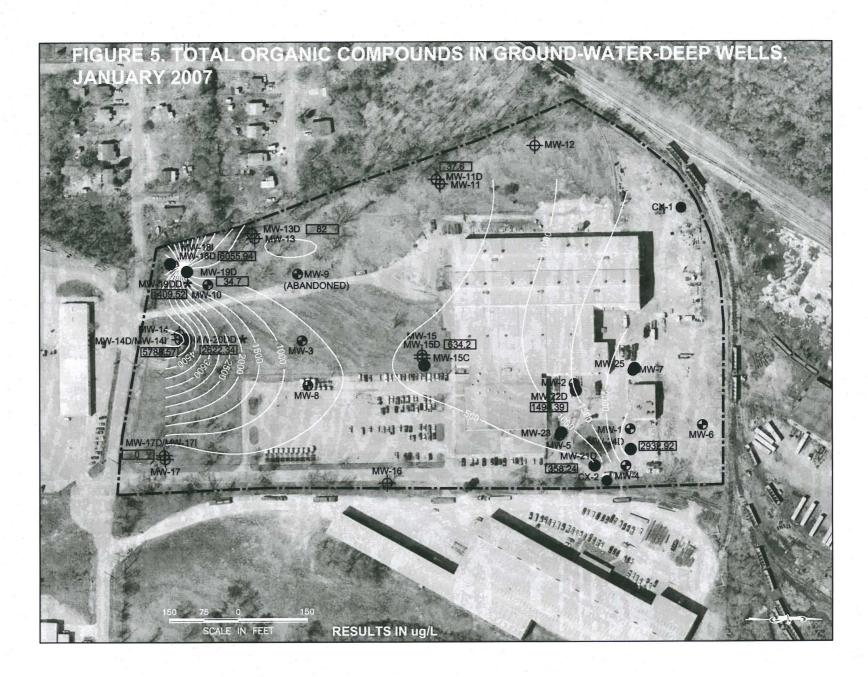
Ground-water analyses indicate that many wells have concentrations of halogenated hydrocarbons above Maximum Contaminant Levels. The distribution of the organic constituents illustrates the source area in the vicinity of the facility operational area in shallow wells and migration and degradation by-products (chemical and biological transformation) in deeper wells, down strike.
